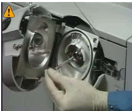
Figure 38 Reinstalling the capillary
