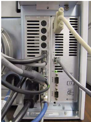
Figure 67 Disconnect the instrument power cable.
