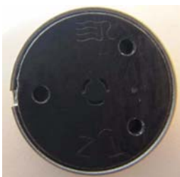
Figure 48 CDS rotor valve in its proper orientation
