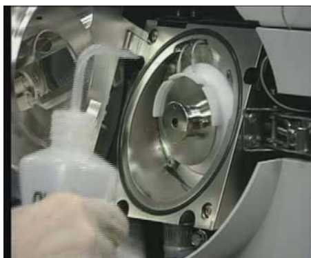
Figure 17 Rinsing the area around the spray shield
