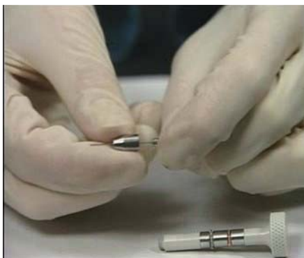
Figure 35 Installing a new needle into the collar
