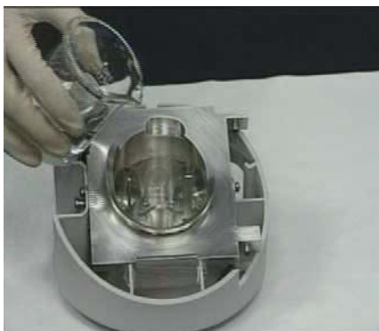
Figure 2 Filling the spray chamber
