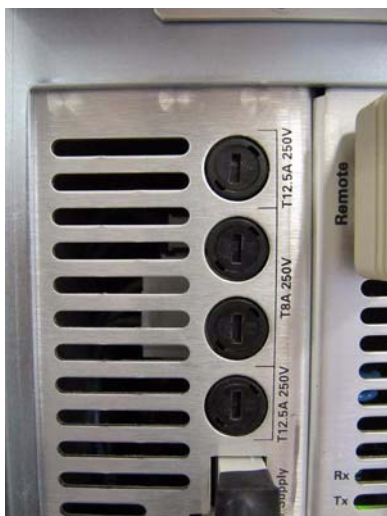
Figure 68 AC Board fuses
