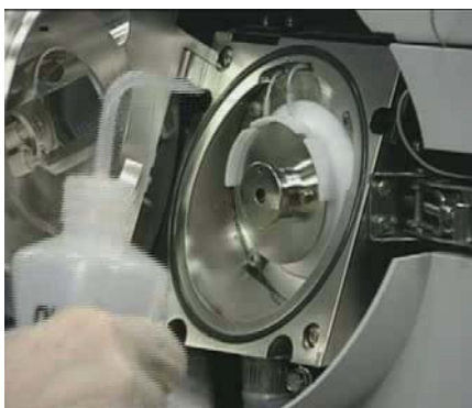
Figure 4 Rinsing the area around the spray shield
