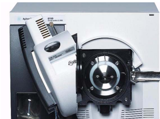
Figure 14 Opened electrospray Agilent Jet Stream Technology spray chamber
