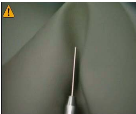
Figure 34 Pulling and twisting abrasive paper along the tip of the needle
