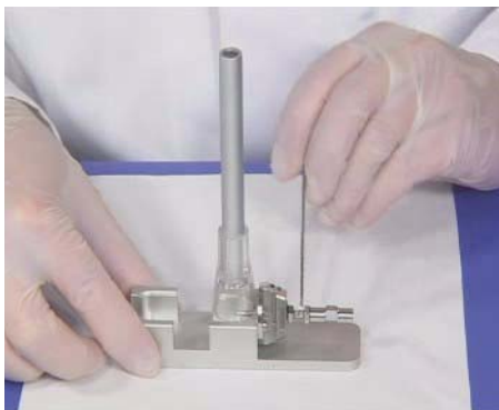
Figure 32 Installing the nebulizer in the adjustment fixture
